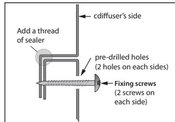
Locates on each side of the duct, two pre-drilled holes help to secur thighten the SRA with the screws provided for this purpose.
